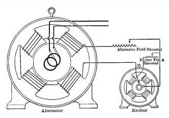
FIG. 54. Diagram of field excitation from separate exciter as used in alternator practice.
